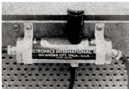
THIS is the coaxial switch which feeds both the off-air and out-of-wire signal to the tv receiver. It is clamped to the back of the set, with the handle up, available to be pushed to "TV" (off air) or "TM" (Telemovies). The assembly terminates in a transformer which corrects for the difference in impedance of the twin lead from the antenna and of the coaxial cable.
